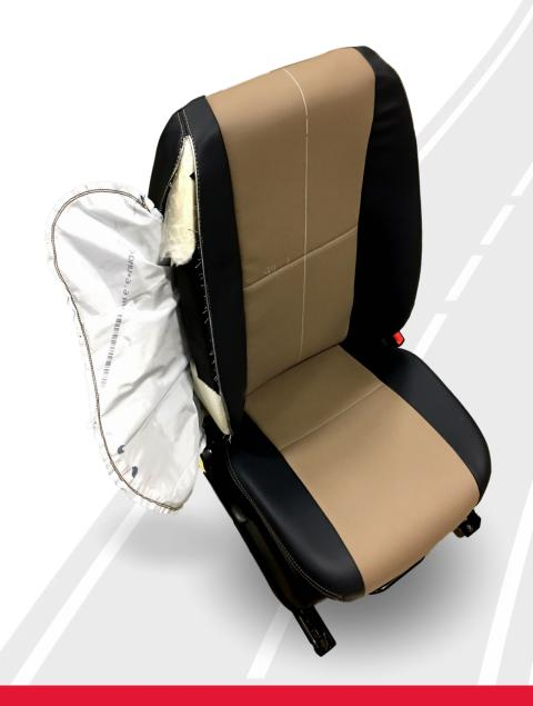
HSM front airbag seat recovers are specifically designed for the van and truck markets to match styling throughout the vehicle.
